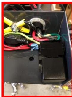
3. Inline fuse. Found inside electrical box. (7.5amp automotive type 2 prong fuse)
