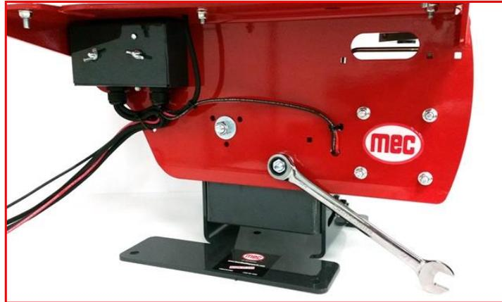
**Step 9** – Adjust the machines tilt by loosening the ¾” nut on the front and rear on the base of the machine, as shown below. Tilt the machine to the desired angle and then retighten both nuts securely.
