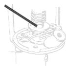
In cases of accidental spilling of powder or shot the MEC 500 can easily be cleaned by merely lifting the column spring approximately  $1\frac{1}{2}$ " and inserting a nail or similar object in hole provided. Lift the shell carrier, remove Primer Seating Assembly and clean.
