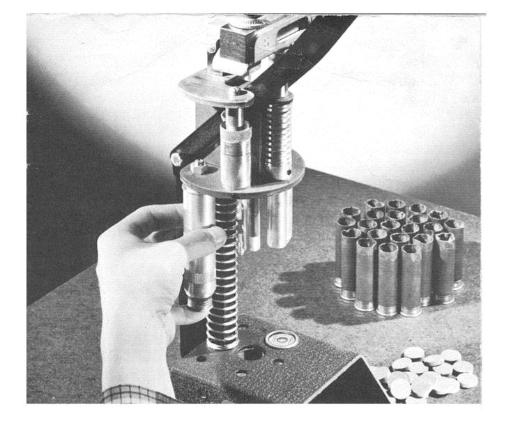
press handle. If shell lodges in the Crimping Sleeve, place the shell with Crimping Sleeve into opening located below ejecting punch and depress handle. This will eject finished shell.
