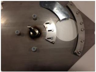
**Step 5: (optional)** Using a 1/2" wrench remove the throwing plates 4 nuts. This will allow you to change the soft fall plate easier than leaving it on the machine. However, you will need to re-set the plate to the throwing arm after removing.
