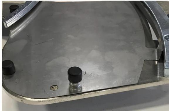
**Step 9: (If you removed the throwing plate) Re-mount the throwing plate with 4-1/2” nuts.** <https://www.youtube.com/watch?v=qPnQpIMGT7E>
