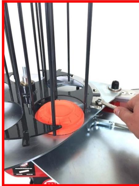
**Step 11:** Reattach carousel in this order. Place carousel on shaft, put on grey spacer, put on silver washer, and then tighten on 3/4" nut. Set carousel tension so you cannot free spin carousel but be sure to not completely tighten carousel to where it locks in place.
