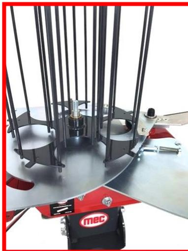
**Step 10:** Using a 7/16” wrench and a midi clay, reset the inner and outer knife edges to appropriate width and height. The height should be set so
